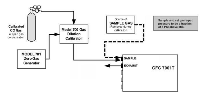
Figure 9-2: Pneumatic Connections – Basic Configuration – Using Gas Dilution Calibrator
